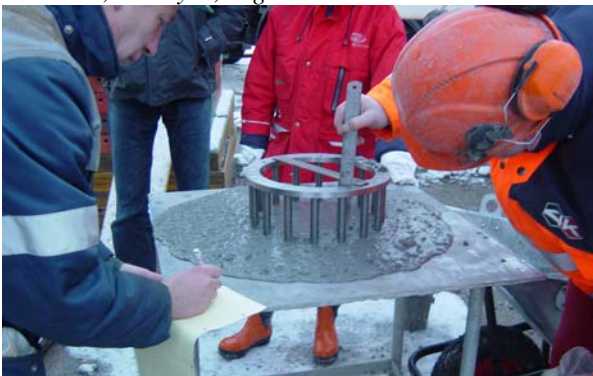
Measurement of fresh concrete properties of fresh concrete of SCC with a J-ring, DR-Byen, Segment 3.
